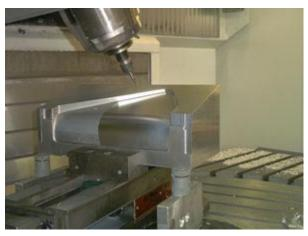
**5th Axis Machining In-Progress**
